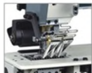
V-008VC-08064/VPL 8 needle half cylinder type used for tape attaching Double chain stitch machine
